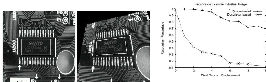
**Fig. 5.** Synthetic experiments: In the left picture the original template image is depicted. The region of interest is overlaid in white. In the middle a perspectively distorted test image is shown. The detected template is denoted with the white rectangle. In the right the results of the detection experiments is plotted.
